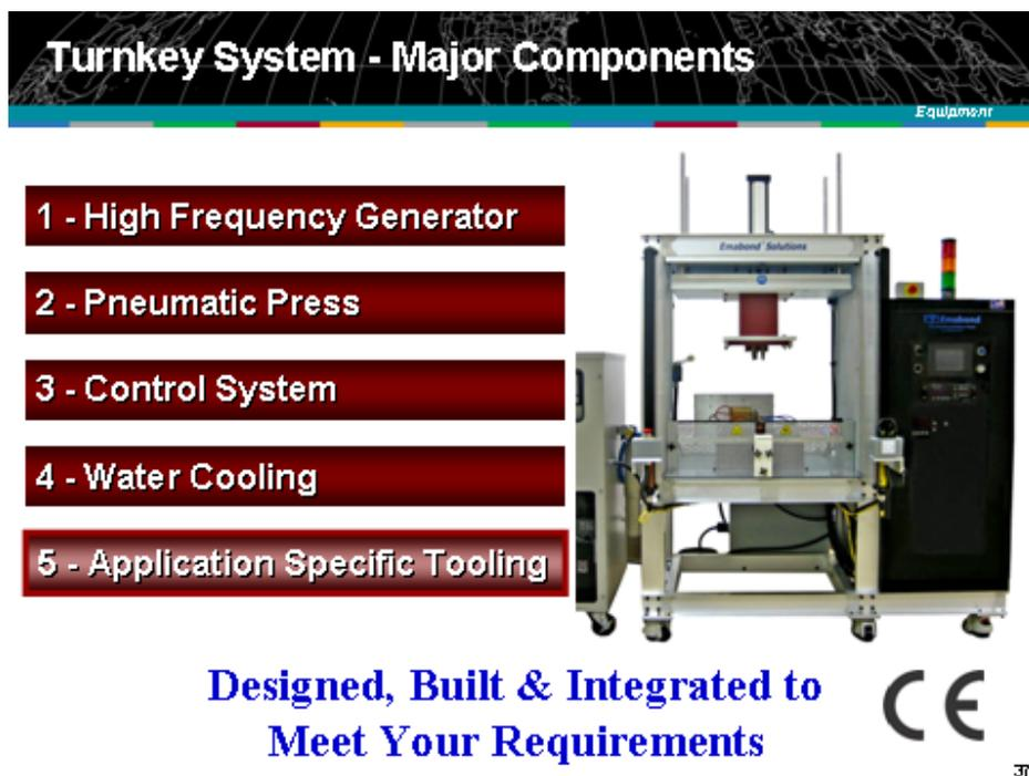
The diagram illustrates the major components of a turnkey induction welding system. It features a central image of the equipment, a list of five components on the left, and a CE mark on the right. The components are:
