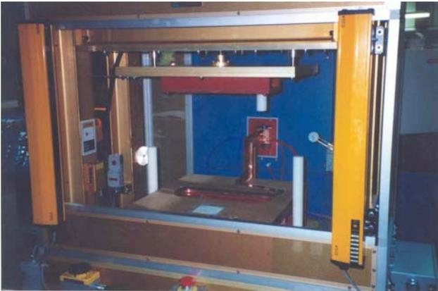
Figure 6 Emabond Welding Machine
