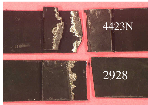
Figure 9 Fracture surface of high strength welds
